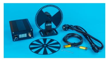
Optomechanical Chopper OMC-1 is designed to modulate a continuous or semicontinuous optical radiation by blocking the radiation beam with an opaque metal wheel that has some slots in it.
