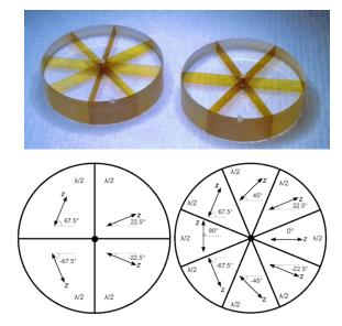
Operating principle of segmented waveplates:
