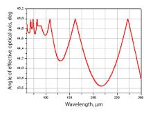
Fig. 3a Angle  $\theta$  of effective optical axis of the APC L/4@60-300  $\mu m$
