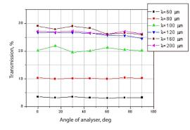
Fig.5 Measured transmission of the APC L/4@60-300  $\mu m$  as a function of analyzer angle  $\beta$
