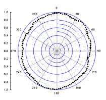
Fig.6a Laser radiation intensity versus analyzer rotation angle in the case of linear polarised radiation passing through the AWP L/A@60-95 μm
