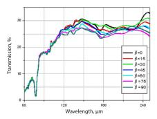
Fig.4 Measured transmission spectra of the APC L/4@60-300  $\mu m$  at different analyzer positions
