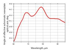
Fig.3b Angle  $\theta$  of effective optical axis of the AWP L/4@60-95  $\mu$ m
