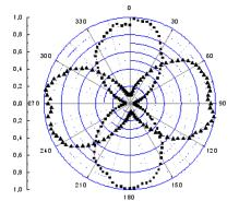
Fig.6b Laser radiation intensity versus analyzer rotation angle in the case of circle polarised radiation passing through the AWP L/A@60-95  $\mu m$
