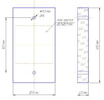
Fig.1 Drawings of the drilled windows
