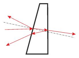
Fig.2 A method to rid the optical system of unwanted reflections with using the wedge
