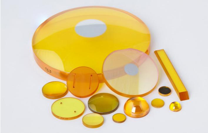
ZnSe, germanium, and silicon are all used in pyrometric applications. However, Zinc Selenide has several advantages over the other two materials. It has a wider transmission spectrum from 0.5 mm to 19 mm (see Fig. 1) and a lower absorption coefficient.
