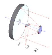
1 – primary element, concave parabolic mirror;
