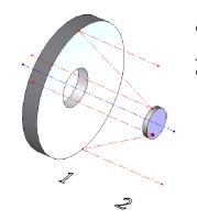
1 – primary element, concave parabolic mirror;
