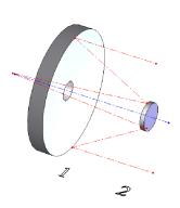
1 – primary element, concave parabolic mirror;
