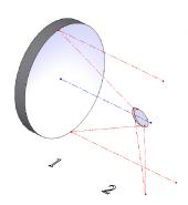
1 – primary element, concave parabolic mirror;
