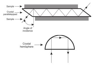
Fig.1 Light propagation through ATR elements
