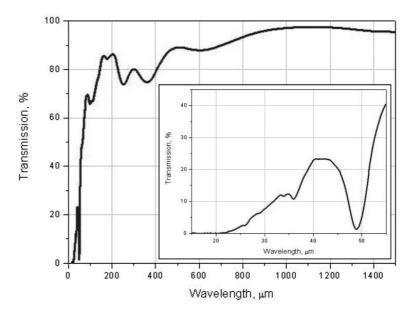
*Fig. 1.* Transmission spectrum of low pass filter with blocking wavelength 21 µm
