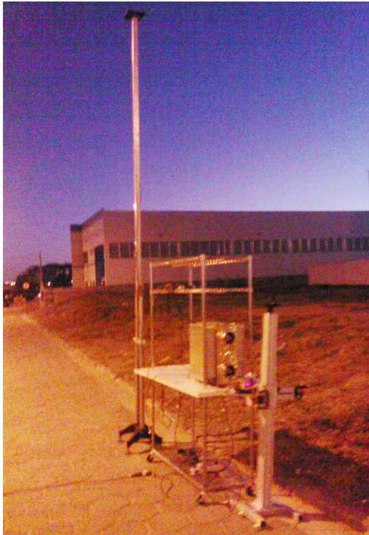
Fig. 12 Realistic operational tests performed with SOLAR-T “on-board” setup, with hot source in front of telescopes, coupled to Iridium antenna at the top of the mast. Results are shown in Fig. 13
