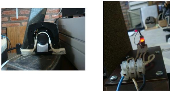
Figure 2. INO camera with TydexBlack THz filter placed in front of the FPA (left). At right the nichrome heated resistor, the 0.15 m concave reflector in the background aligned to form its image in the camera FPA (located behind the protecting surface, at the left of the picture).
