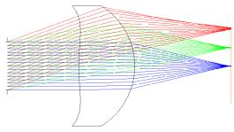
Fig. 1. THz aspherical f-theta lens
