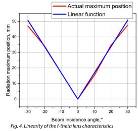
THz aspherical f-theta lenses are manufactured to customer specifications. To perform the calculation it is necessary to specify diameter, wavelength, focal length, scanning angle, scanning field and input beam dimensions.
