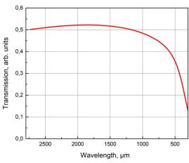
Fig. 3. Transmission spectrum of a 40 mm thick f-theta lens along the axis
